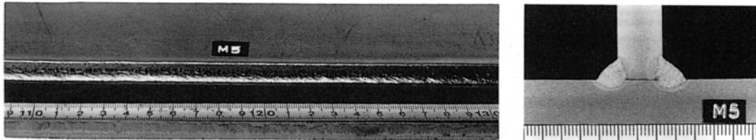
Fig. 2 Bead appearance and cross-sectional view of a fillet weld (MX-200, 1.2 mmØ, 280 Amp. 28-32 Volt, 50 cm/min)
