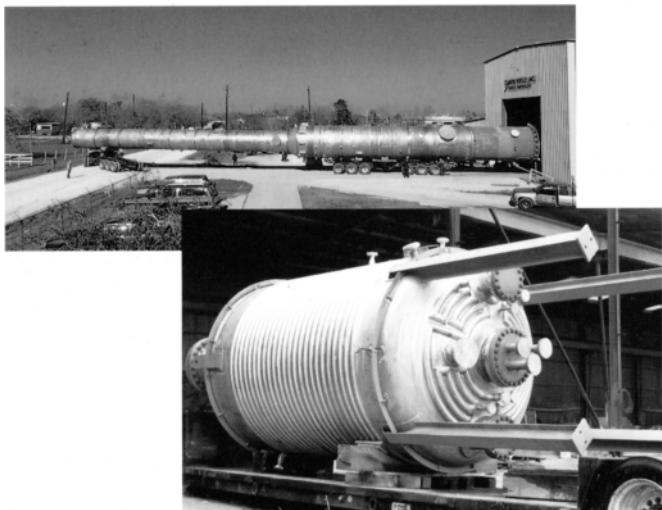
Vessels for cryogenic service, welded with DW-308L
