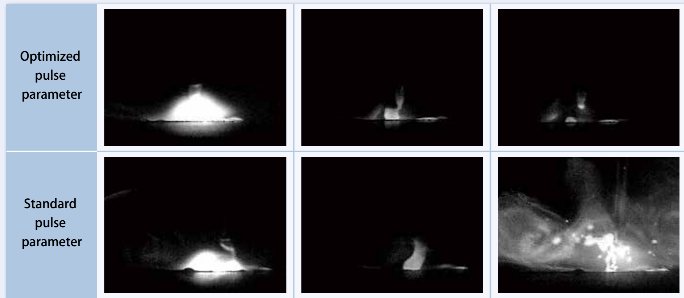
Figure 8: Droplet transfer with optimized and standard pulse parameter
