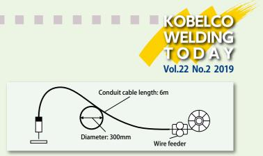
Figure 5: Schematic drawing of wire feeding test
