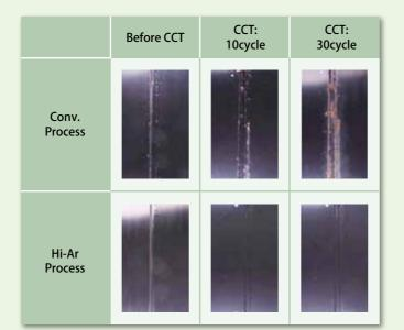
Figure 10: Comparison of corrosion resistance between conventional and Hi-Ar processes
