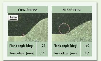
Figure 11: Comparison of toe shapes
