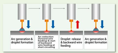
Figure 3: Wire feeding control method
