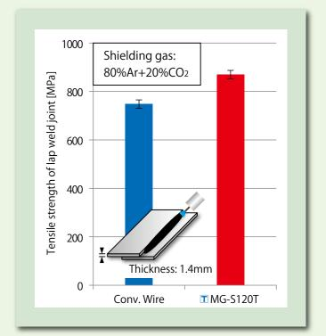
Figure 1: Comparison of tensile strength of lap joints welded with conventional (JIS Z 3312 YGW16) and T MG-S120T wires on 980MPa class steel sheets
