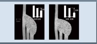
Figure 3: Examples of gap resistance evaluation with **PMX-T430Nb**
