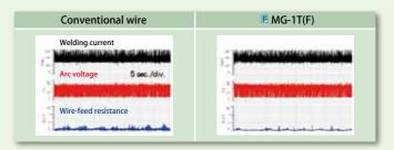
Figure 6: Time variation of welding current, arc voltage and wire feed resistance between a conventional wire and **F** MG-1T(F)
