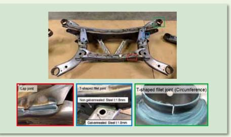
Figure 13: Appearance and welds of suspension cross-members
