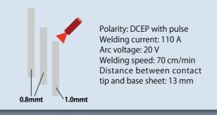
Figure 2: Welding condition
