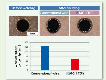
**Figure 4: Comparison of wear at the contact tip** \*\*One hour continuous welding at 200A-25V, 100%CO<sub>2</sub> gas
