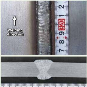
Note: 1. Welding position: Vertical upward(3G) 2. Current:160A (DCEP) 3. Voltage: 26V 4. Shielding gas: 80%Ar-20%CO2 5. Travel speed:15cpm
