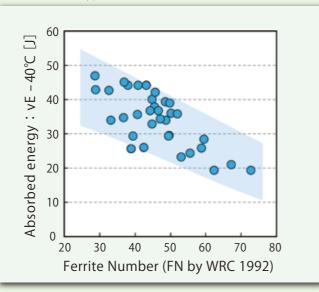
within a range from 30 to 65. In addition, because the weld metal is less corrosion resistant than the base metal, which is produced through a process of thermal refining, it is designed to hold slightly higher amounts of alloying elements (higher PREW) than the base metal. The Ni content of the weld metal is also designed to be higher than that of the base metal in order to optimize the ratio of austenitic and ferritic grains under as-welded conditions in many cases. <sup>(2), (3)</sup>
