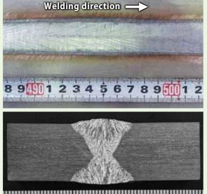
Note: 1. Welding position:Flat(1G) 2. Current: 450A (DCEP) 3. Voltage: 32V 4. Travel speed: 35cpm 5. Pass sequence: 1 pass each/1st and 2nd layer 6. Wire size: 2.4 mm dia **5** Selection of welding consumables
