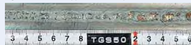
Figure 2: Back bead appearance in 1G position
