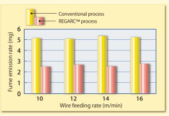
It is clear that the REGARC<sup>TM</sup> process generates nearly half the amount of fumes compared with the conventional process.
