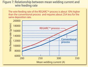
The wire feeding rate of the REGARC<sup>™</sup> process is more than 10% higher than that of the conventional process. Because the pulsing welding current of the REGARC<sup>™</sup> process is higher than that of the conventional process, resulting in higher Joule heat, the deposition rate (and overall efficiency) of the REGARC<sup>TM</sup> process is higher for any amount of welding current (mean value) used.
