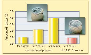
When spatter sticks to the inside of a nozzle, shielding may be reduced, resulting in poor mechanical properties as well as welding defects such as weld metal porosity. For this reason, robotic welding incorporates automatic nozzle cleaning and nozzle exchanging in order to maximize operation time.
