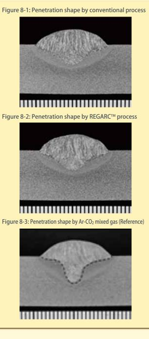
Even though the mean welding current of the REGARC<sup>™</sup> process is lower than that of the conventional process, similar penetration is obtained (Figures 8-1 & 8-2) because of the higher peak current of the REGARCTM process. Hence, it can be seen that sound welding can be performed despite lower heat input.
