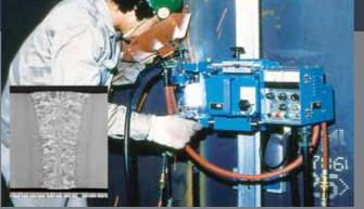
front side electrode is connected in DC-EP polarity but the root side electrode, in DC-EN.
