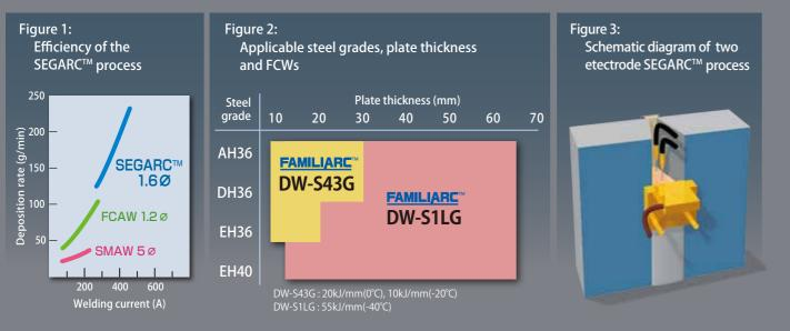
In case of applicable range up to 80 mm thickness, a second electrode has been added to the standard apparatus. A schematic diagram with two electrodes is shown in Figure 3. The procedure is nearly the same
