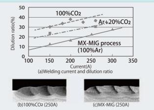
It is clear that the MX-MIG process allows low dilution overlay welding even with high current/high deposition welding and thus reduces the number of welding passes as well as working time.
