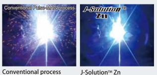
Gas : Ar+20%CO2 Diameter:  $1.2mm\Phi$ Pulse wave: Conventional rectangular
