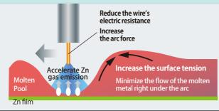
MIX-Zn solid wire was developed to optimize surface tension as well as to apply a higher current with the same deposition amount by reducing the wire's electric resistance.
