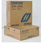
SMAW in general, resulted in poor notch toughness. DW-A80L (AWS A5.29 E111T1-GM-H4) provides a solution by controlling the oxygen content in the flux while maintaining high notch toughness. The diffusible hydrogen content with DW-A80L is around 2.5ml/100g, as shown in Table 5, an extremely low level for a rutile type FCW.
