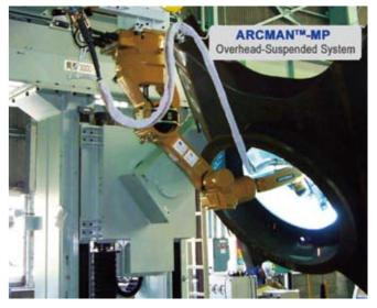
In this case, internal cabling could prevent interference between the torch cable and workpiece, allowing the teaching operation to be easily carried out. Also the cable-integrated model allows off-line teaching to be conducted on a personal computer because no unpredictable cable movement can occur.
