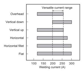
Figure 2: Proper welding current ranges for individual welding positions and versatile current range for positional welding (DW-100, 1.2Ø, CO<sub>2</sub> shielding).
