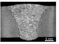
Figure 12: Typical macrostructure of EGW weld joint by SEG-ARC process
