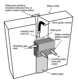
Figure 10: Principles of the SEGARC process for EGW of vertical joints of 9-25 mm in thickness and 2-6 m in length.
