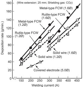
Figure 1: Deposition rates of covered electrodes, solid wires, rutile-type FCWs, and metal-type FCWs as a function of welding currents.
