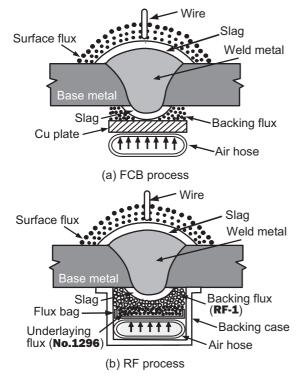
Figure 2: Principles of FCB and RF processes for plate-toplate one-sided SAW.
