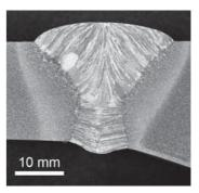
Figure 3: Macrostructures of weld joints made by one-sided SAW (top: FCB process; bottom: RF process)
