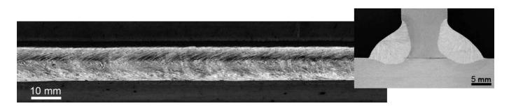
Figure 2: Bead appearance and macrostructure of MX-200E fillet weld made on inorganic-zinc-primer-coated steel fillet joint.
