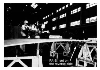
Figure 6: FAB process being used on a curved work with **FA-B1** attached on the reverse side of the work.
