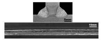
Figure 8: Typical bead appearance and macrostructure of **MX-200H** (1.6 mm $\emptyset$ ) fillet weld made by the TOP process on a primer coated steel plate (CO<sub>2</sub> shielding; inorganic zinc primer of approx. 20 µm thick.; travel speed of 150 cm/min.)
