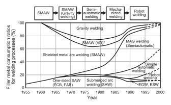
Figure 1: Changes in filler metal consumption ratios for individual welding processes used by the shipyards of Japan (VD: vertical downward position) [Ref. 3].
