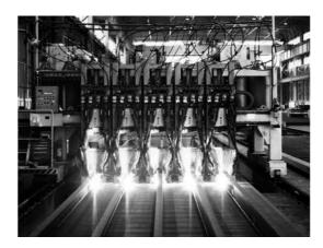
Figure 9: Twin tandem welding of five longitudinals onto one panel by using **MX-200H** flux-cored wires.
