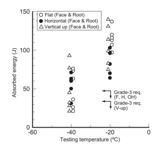
Figure 1: Absorbed energy obtained in Charpy impact testing of weld joints (Wire: DW-100E, 1.2mmØ; Base metal: SM490A, 25mm thick., single-V groove; Welding current: 180-280A; Arc voltage: 24-30V; Shielding gas: 100%CO<sub>2</sub>; Welding position: flat, horizontal, vertical up; Backing: FB-B3).
