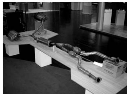
An automotive exhaust system flux-cored arc welded with MXA-430M
