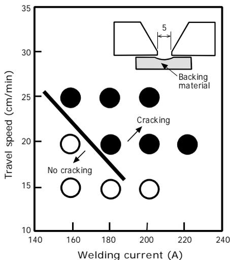
Figure 7: Hot crack susceptibility of DW-329AP root pass weld metal in one-side FCAW with FBB-3 backing
