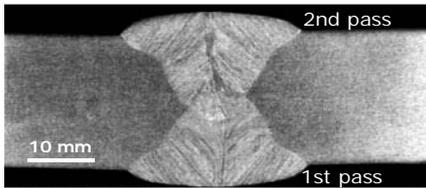
(1) The 1st or backing pass was water-cooled when the 2nd or final pass was welded to prevent reheat embrittlement of the 1st pass weld metal.
