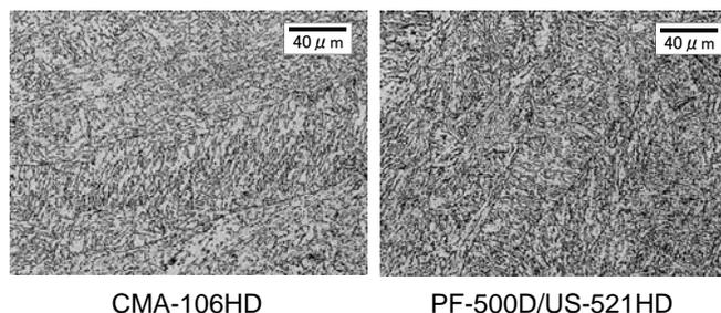
Figure 2: Fine bainitic microstructures of CMA-106HD and PF-500D/US-521HD weld metals after PWHT (705°C x 7h)
