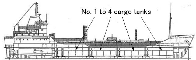
Figure 2: A chemical tanker's cargo tank sectioned by several transverse bulkheads
