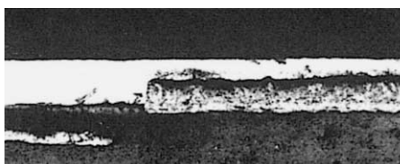
Photo 1. Self-peeling slag removal of DW-100
