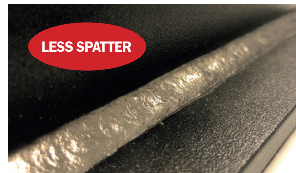
Horizontal Fillet (PB) Welding
